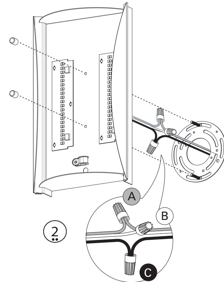
A: Copper ground wire to ground wire - If you only have two wires coming from the electrical box, connect the fixture's copper wire to the green ground screw on the mounting plate.
